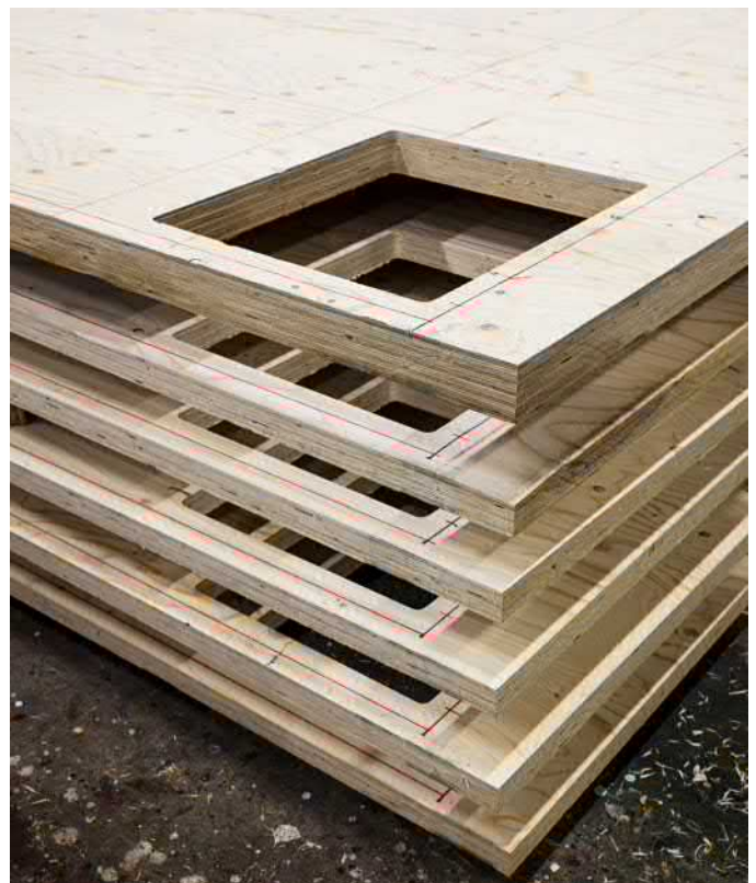
Figure 1.48. Holes in LVL panels.
