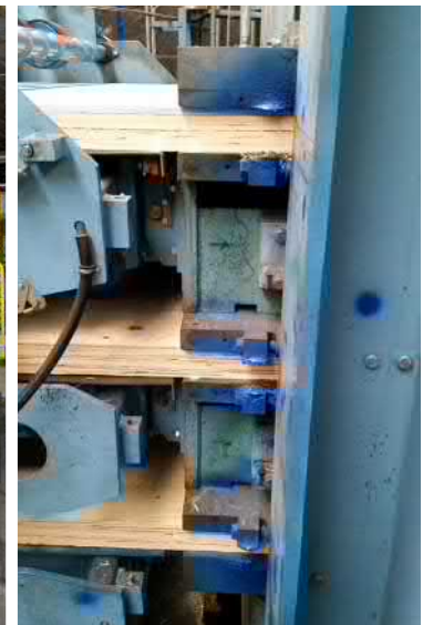
Figure 1.43. Feeding LVL billets into 3-level hot press.
