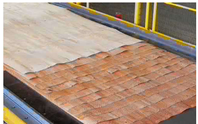
Figure1.40. Staggered layup ahead of the pre-press.
