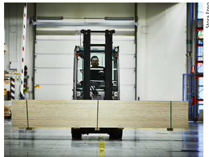
Figure 3.3. Use wide enough forks when moving LVL packages with forklift to avoid damage.
