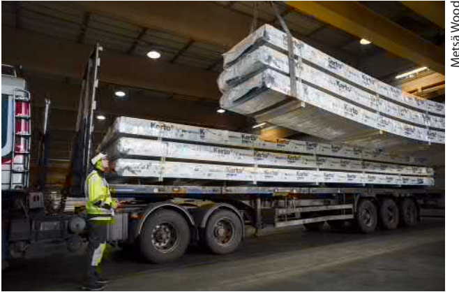
Figure 3.2. Loading LVL packages with an overhead crane for truck transport.
