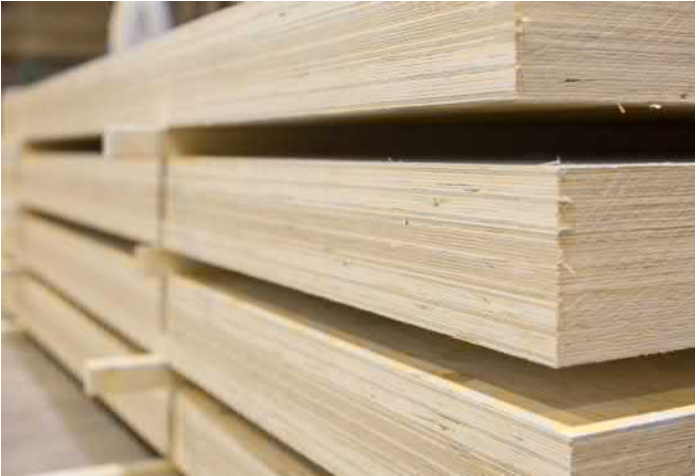
Figure 3.4. Storage of LVL packages
